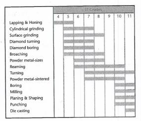
**10.36** International Tolerance Grades Related to Machining Processes. *Reprinted from B4.2-1978, by permission of The American Society of Mechanical Engineers.* All rights reserved.
